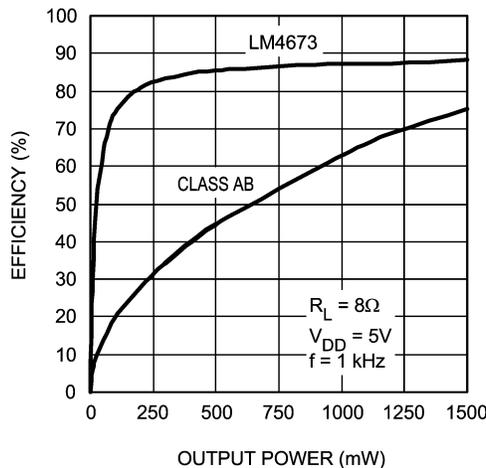
FIGURE 1. LM4673 vs. Class AB Efficiency
