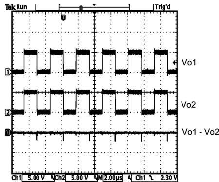
**FIGURE 6. In Phase Switching**
