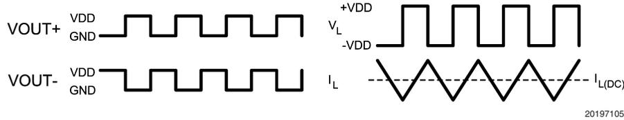
**FIGURE 5. Conventional Class D Switching**
